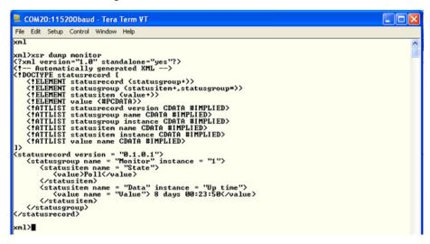
For XML we start at the root Command Line Interface, type "xml", then "xsr dump monitor".
